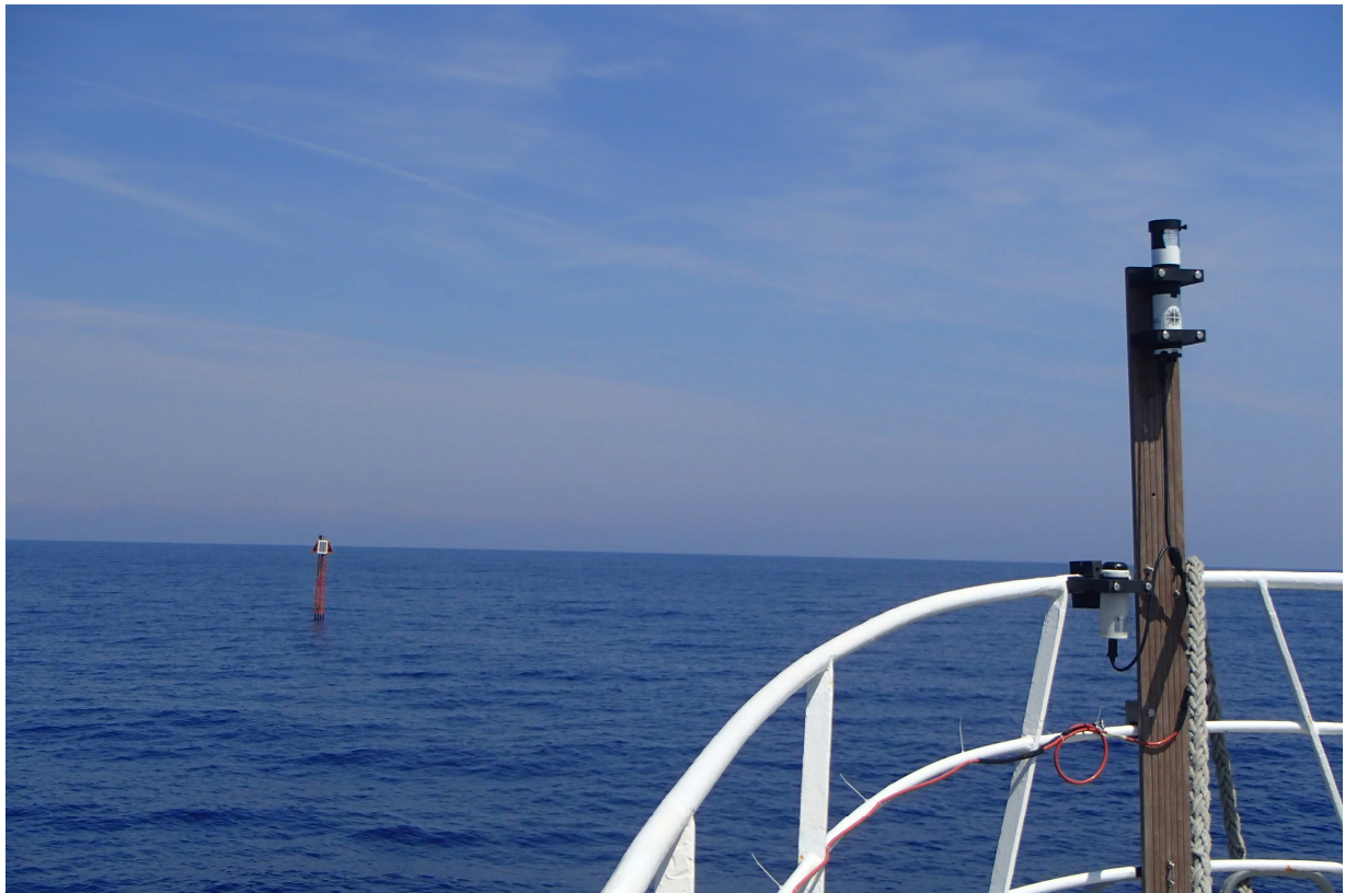
On the right of the image, at the forward deck of the R/V Téthys II : the C-OPS reference radiometer (measuring above-surface downward multispectral irradiance, E_d(0^+) ). The BOUSSOLE buoy appears on the background.
